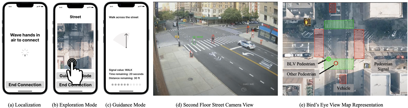
Figure 1: Overview of the street camera-based navigation system. Blind and low-vision (BLV) pedestrians use the smartphone app (a–c) to interact with the street cameras (d–e) in receiving precise and real-time navigation assistance. The system (a) localizes the BLV user by asking them to wave one hand, offering them the ability to (b) explore the environment layout, and then (c) guides the user to their destination while avoiding obstacles and veering off track, and assisting with crossing streets.
